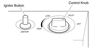
Figure 16 - Control Knob In The OFF Position
